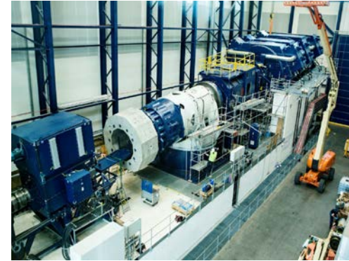
Full scale test facility for the entire power train Aarhus, Denmark
